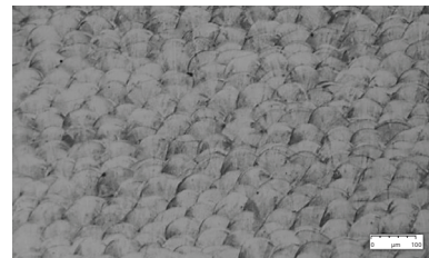
Microstructure after stress relief
