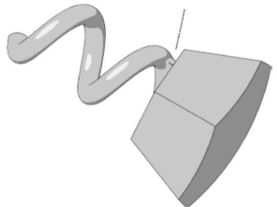
The key to coil springs is the junction between the spring and what it's connected to. Make sure you apply as much fillet to the acute apex as your design will allow.
