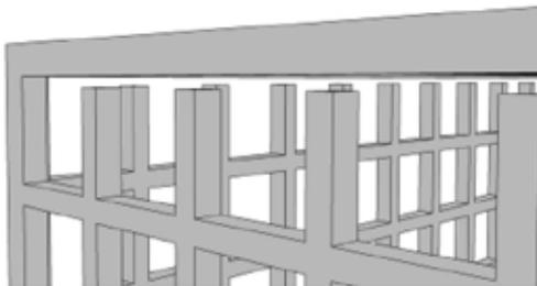
In applications requiring additional post processing, such as sterilization for surgical use, the batch can transition through the various processes within the cage. To remove the parts consider CAD modeling in hinge doors, apply snap-off regions or, as in this example, connect the lid with the four corner posts that can be cut off with wire snips.
