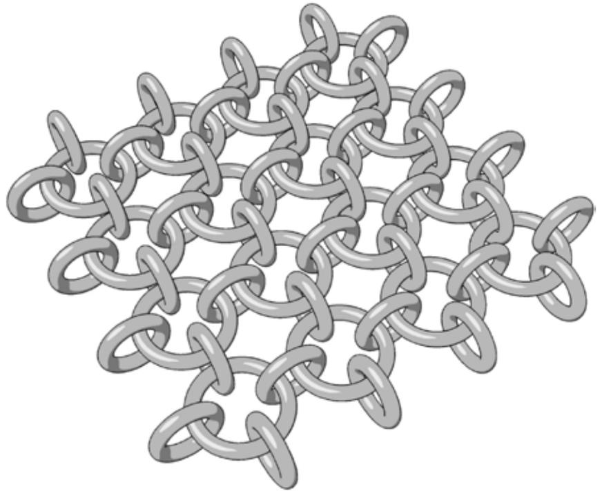
Invest time in getting a single link optimized before array duplication. Consider using a polygon instead of the circle to speed up link duplication and manipulation in CAD.
