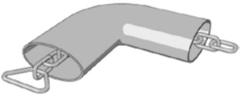
Consider CAD modeling in a chain through the duct. When finishing, a quick pull of this chain through the duct will clear an open channel for the bead blasting media to get a good cleaning velocity in the duct.
