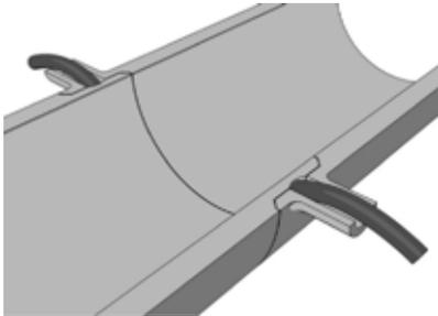
Above cross section shows glue (dark) getting sucked into radial cavity through access ports.
