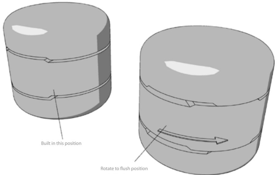
To solve this, one approach is to apply a form where the hinge rotates into a flush position. Generous tolerances in excess of 1mm can be applied in the disengaged state for building, while tolerances of approx 0.05mm will enable a flush intimate stable interaction in the engaged functional range of the rotation.
